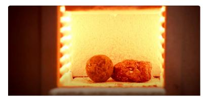
In the second, the temperature of the two bodies has reached the same temperature as that of the oven. The oven, the iron ball and the stone radiate in exactly the same way.
